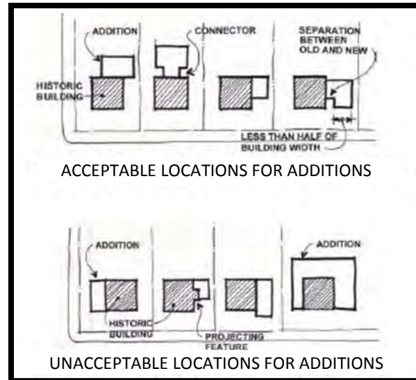
FIGURE 41: EXAMPLES OF ACCEPTABLE AND UNACCEPTABLE ADDITION LOCATIONS.
